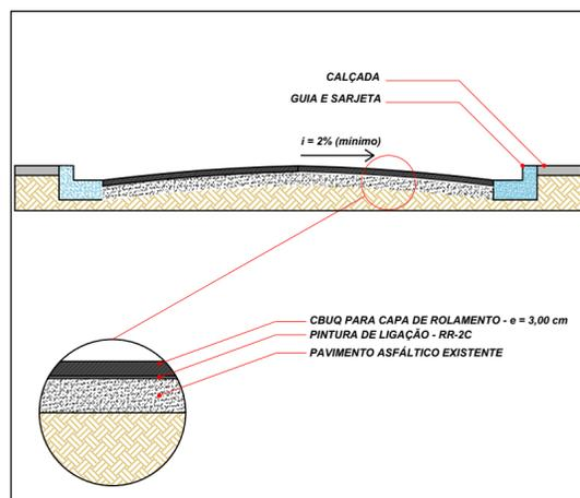
DETALHE CAMADAS DO RECAPE ASFÁLTICO
